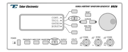
Figure 3-10. Selecting a Trigger Mode
