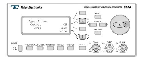
Figure 3-13. Enabling the SYNC Output
