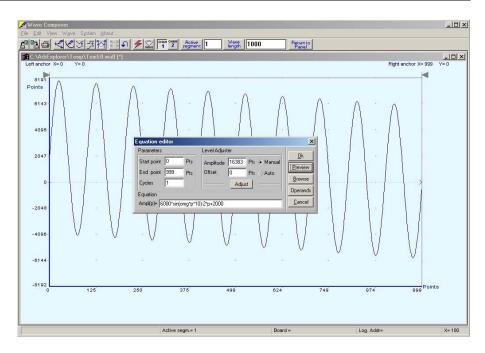
Figure 5-21. Using the Equation Sample to Combine Two Waveforms
