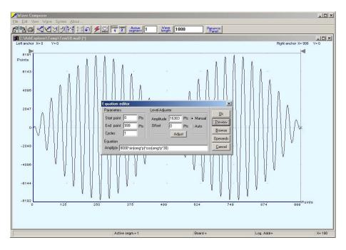
Figure 5-22. Using the Equation Editor to Modulate Sine Waveforms.
