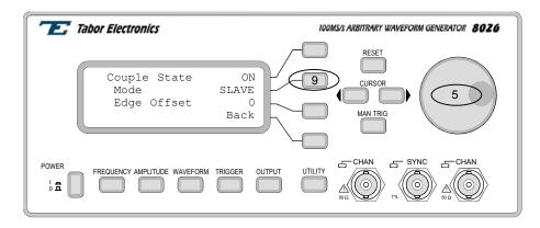
Figure 3-28. Setting Master/Slave Parameters
