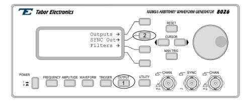
Figure 3-12. Selecting the SYNC Output Menu
