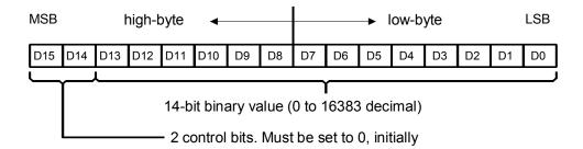
Figure 4-2. 16-bit Initial Waveform Data Point Representation
