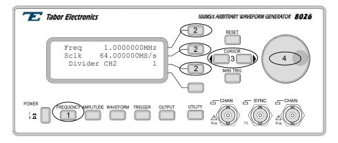
Figure 3-6. Modifying Frequency, Sample Clock and Channel 2
