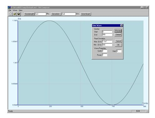
Figure 3-22. Using ArbExplorer to Generate Arbitrary Modulating Waveforms
