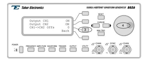
Figure 3-26. Adjusting Phase Offset Between Channels
