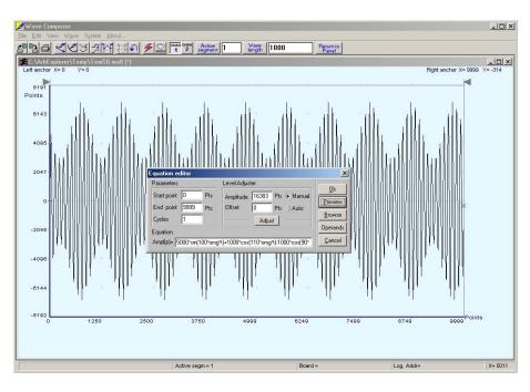
Figure 5-25. Using the Equation Editor to Build Amplitude Modulated Signal With Upper and Lower Sidebands
