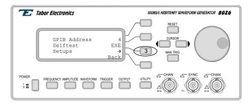
Figure 3-32. Selecting Arbitrary Waveform Segments
