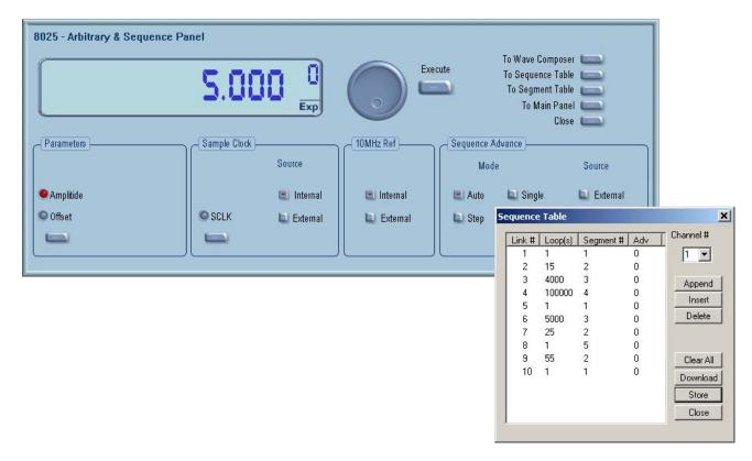
Figure 3-33. Using ArbExplorer to Generate Sequences
