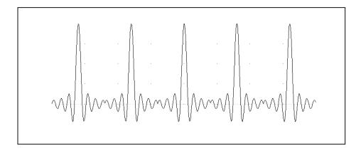
Figure 1-6a, Segment 1 – Sin (x)/x Waveform
