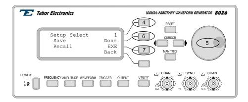
Figure 3-30. Saving and Recalling Setups
