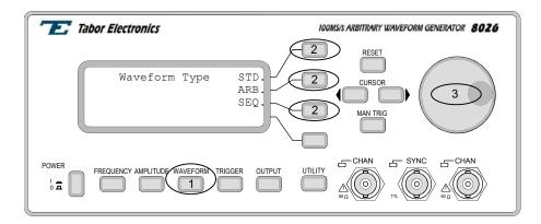
Figure 3-5. Selecting Waveform Type
