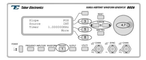
Figure 3-11. Programming trigger parameters
