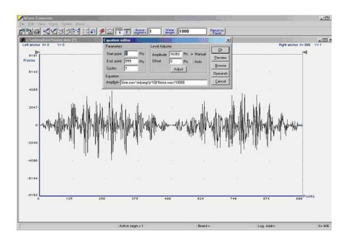
Figure 5-26. Combining Waveforms Into Equations
