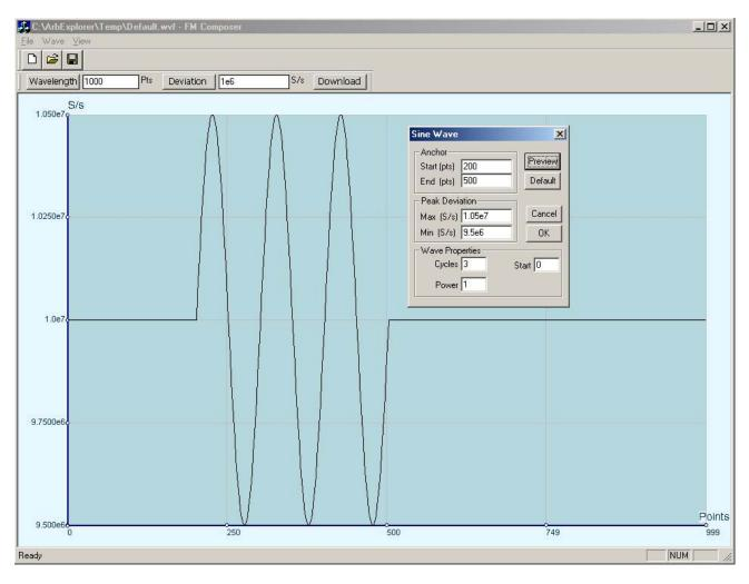
Figure 5-19. An Example of Generating Modulating Sine From the Built-in Library.
