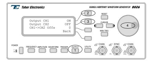
Figure 3-4. Enabling the Outputs
