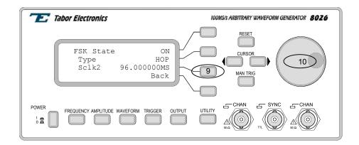
Figure 3-23. Adjusting FSK Parameters
