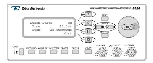
Figure 3-24. Adjusting Sweep Parameters
