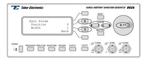
Figure 3-14. Modifying the SYNC Parameters
