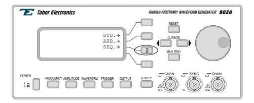
Figure 3-34. Selecting Sequenced Waveforms
