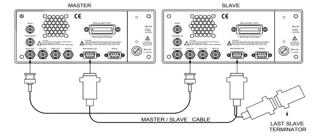
Figure 3-27. Wiring Diagram Master to Slave
