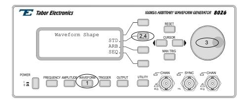
Figure 3-8. Selecting Standard Waveform Shape
